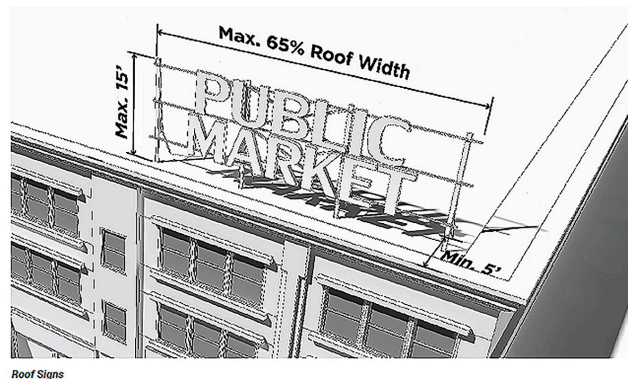
Fig. 32. Typical Diagram from TOD Sign Regulations Sign regulations in any zoning ordinance are usually cumbersome and often arbitrary. This ordinance benefits from the use of clear drawings to illustrate the range of signs that are wanted, not prohibited. Signs can be a source of great creativity, and ordinances should aim to spur innovation and artistic creativity. Image courtesy of City of Charlotte.
