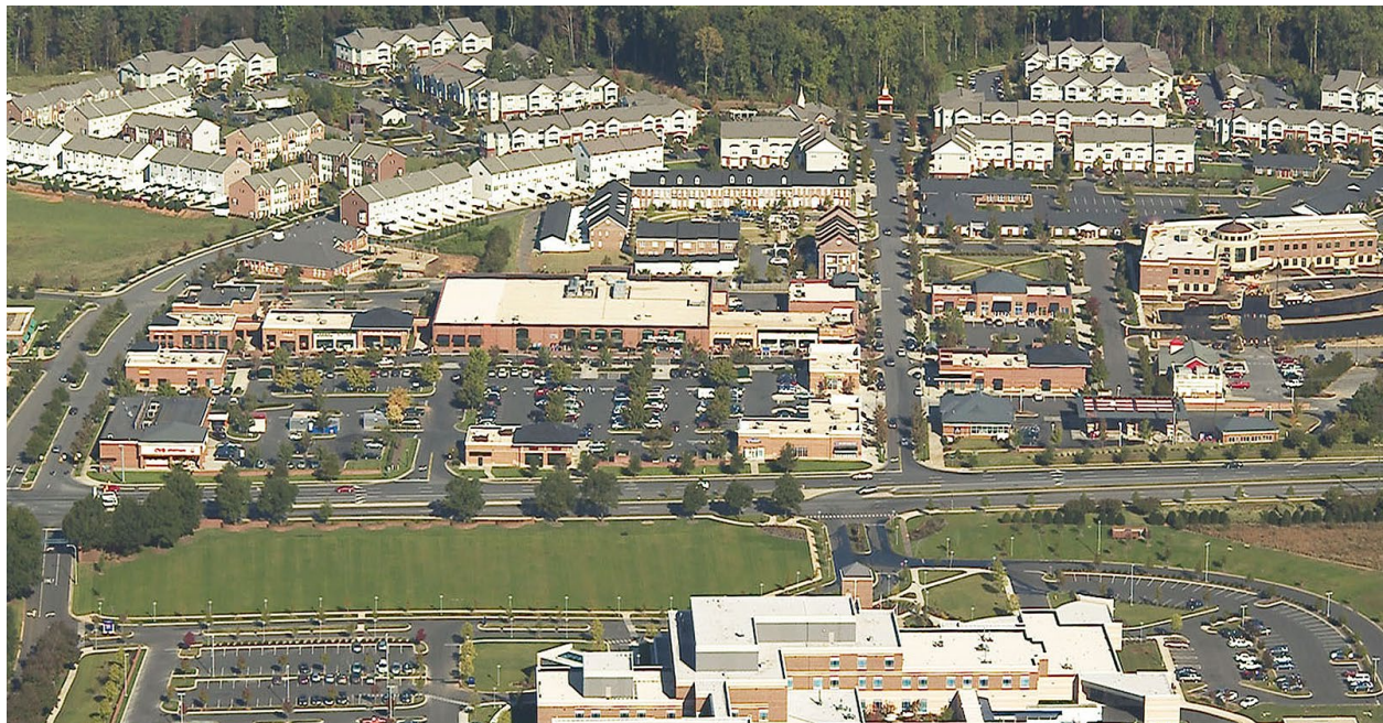
Fig. 18. .Mixed-Use Center with Public Streets. Rosedale Commons, Huntersville, NC. The town's form-based zoning code (adopted in 1997) required all buildings to front directly onto public streets, not parking lots. Illustration courtesy of the Town of Huntersville, NC
