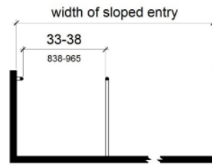
Figure 11B-1009.3.3 Handrails for Sloped Entry
