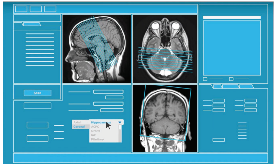
Figure 1. GE Healthcare’s AIRx™ automatically aligns MR scans for better diagnostic imaging.
