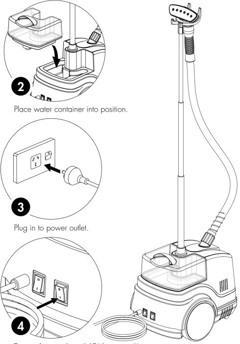
Turn on by switching 'I/O' button to 'I' position. For maximum steam strength, set 'I/II' to 'II'.
