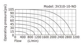
The data in flow rate chart are obtained from AirTAC lab.
