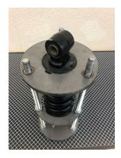
3. Install washer and nuts to top plate and snug against shock pre-load adjuster as seen in the picture. Tip: install setup in vise as seen in picture to hold steady while working.
