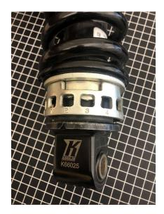
16. Once shock is installed back onto the bike the pre-load can be adjusted as needed.
