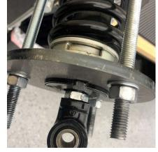
6. You can use a deep socket with extention to hold shock end while loosening locknut. You can also put shock end in vise and loosen locknut. Whatever works for you! Remove shock end from the shock rod. If theshock rod turns you can run the locknut to end of threads on the rod and hold while unscrewing the shock end. Note: Shock pictured is external pre-load adjuster style.
