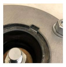
12. Remember to use threadlocker. Tighten the locknut and then align tab with notch. You are now ready to release compression of the spring. Keep the tab and notch in alignment as the spring decompresses making sure the tab falls into place into the notch and the tool's top plate can move freely past and is not binding on pre-load adjuster cup.
