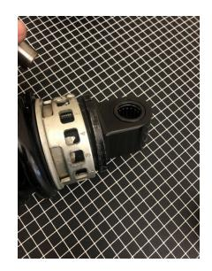
15. After lubing the bearing, the bushing slides right in. Bushing installed and shock is ready to go back onto the bike.
