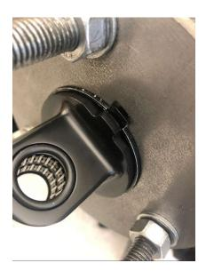
WARNING! Keep fingers away from pinch points in case something is not correctly aligned. Compress spring again enough to align parts. If parts move when under pressure and finger is in the way, you will get hurt so be extremely careful!
