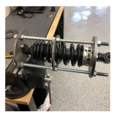
4. Carefully tighten nuts evenly 1-2 turns maximum at a time until the locknut is exposed.
