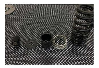
8. Remove the top plate from the tool and remove the spring to get to the upper spring seat. The spring seat on left is replaced with the Kodlin part on the right which is included in the kit.
