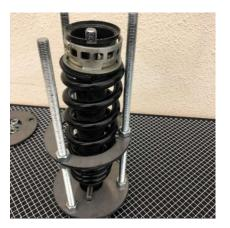
11. Now install top plate and make sure plate is centered around top of the adjuster evenly. Align notch with eyelet on shock end at bottom of picture and gap in cup lines up with notch in plate. Now evely tighten the nuts 1-2 turns a time until you can install the Kodlin Shock end all the way down onto the threads of the shock rod.
