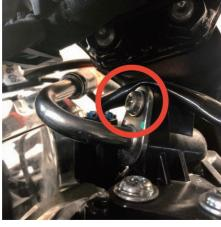
5. Carefully grind off the stock hose clamps, remove the fuel line, and replace it with the clamps and fuel line that are included with your new Kodlin tank
