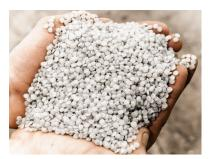
Every milk bottle is ground, washed, melted and cooled to produce purified plastic pellets which are tested to maintain the highest quality control standards.
