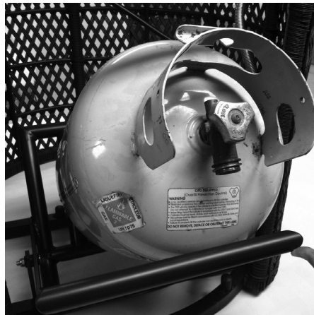
Fig. 17 Place LP tank in cradle. Lift cradle slowly until tank is upright.
