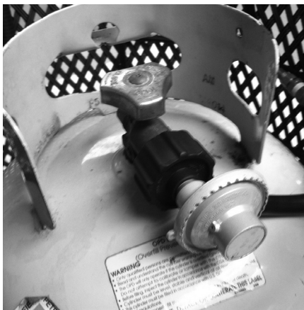
Fig. 19 Ensure all connections are tight and leak free.
