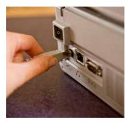
Connect the TD-4100N to a nearby network point, so machine can be sited wherever the labels are required
