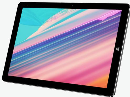
A full metal unibody design gives He10-W+ the weight of only 522g and thinness to only 8.8mm. Delicate CNC and anodic sandblast oxidation processes provides extra premium texture.
