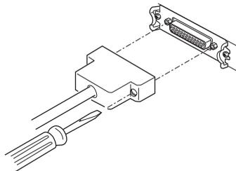
3. Insert the other connector firmly into the interface port of the host computer.
