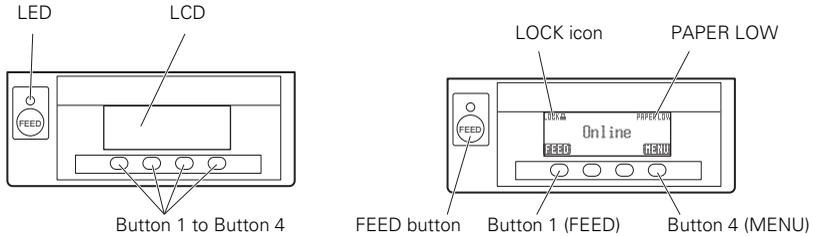
Examples are shown in the diagram of the LCD above on the right.
