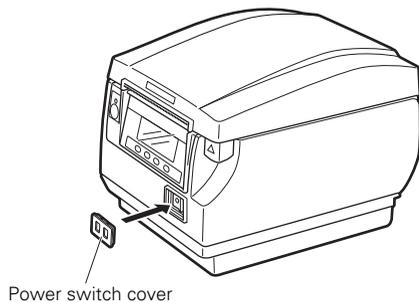
Put a screwdriver or other pointed object into the grooves on the power switch cover to remove it.
