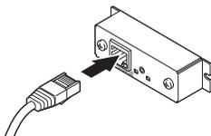
3. Connect the other connector to a hub, router, or similar device.
