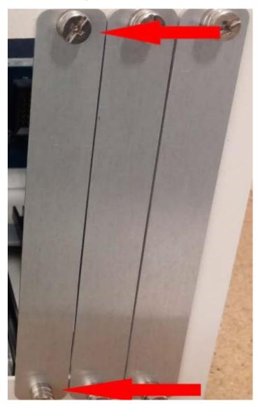
2. Slide card down guide rails into socket:
