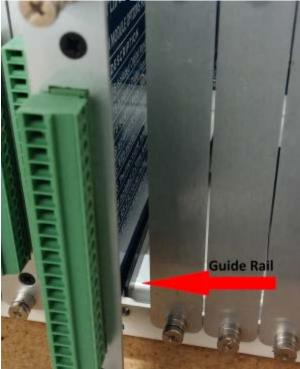
3. Tighten screws on top and bottom of bracket to securely mount the card.
