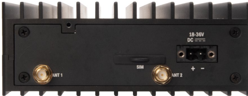
(1) 18-36VDC input with Locking 2 POS Connector (2) SMA for Wi-Fi 6E Antennas
