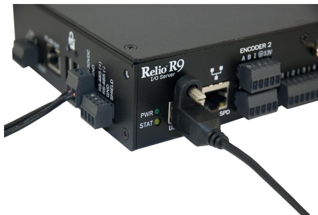
Figure 2 - TR123 tinned leads and Type B USB connector.
