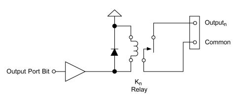
In the above circuit diagram, Outputn is one of the two Output Pair Pins from the table labeled Output Ports Pin Assignments. Common is the other pin listed in Output Pair Pins. Since this is an isolated output, the polarity is not important.
