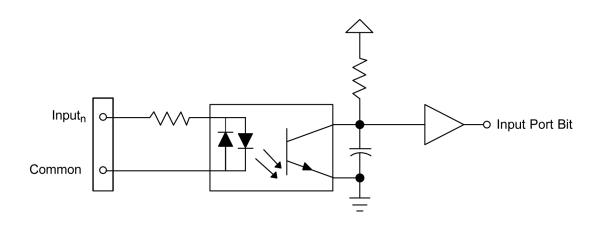
In the above circuit diagram,  $Input_n$  is one of the two Input Pair Pins from the table labeled Input Ports Pin Assignments. Common is the other pin listed in the Input Pair Pins entry. The polarity of the pair does not matter.
