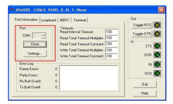
• Click the 'Settings' button to open the COM Properties menu. Change your parameters to 9600 bits per second, 8 data bits, no parity, 1 stop bit, and no flow control, as pictured below.
