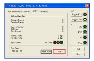
• If the COM port is working properly, the green light will glow, and the Transmit Frames and Receive Frames will increase. The Tx and Rx Data Rates will show the calculated data rate. (Pictured below)
