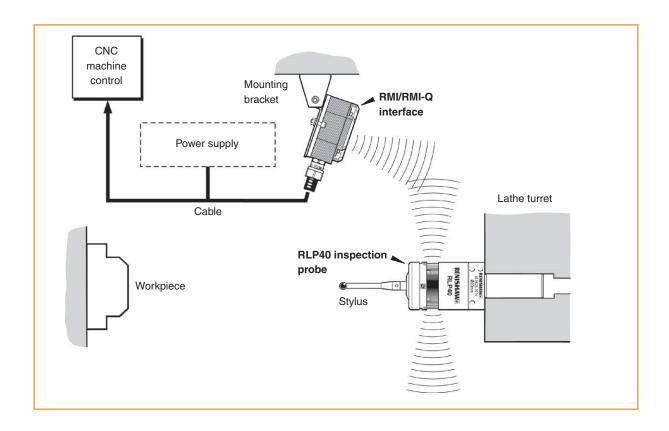
Radio transmission does not require line-ofsight and will pass through very small gaps and machine tool windows. This allows easy installation, either inside or outside the machine enclosure.
