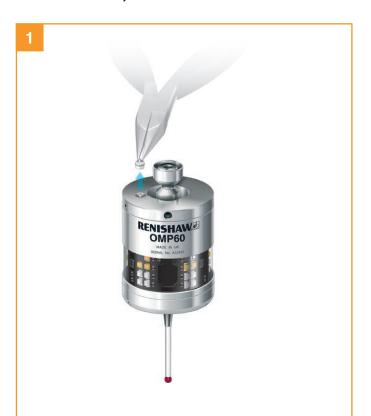
**NOTE:** In instances where the OMP60 is to be used with a shank switch, it will be necessary to remove the plug from the rear of the probe using pliers. This should then be substituted with the bobbin (A-4038-0303).
