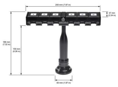
Based on the industry standard range of MCR20 rack systems, TCR20 securely stores modules for rapid automatic changing, protecting mating surfaces from any airborne contaminants within the working envelope of the machine.
