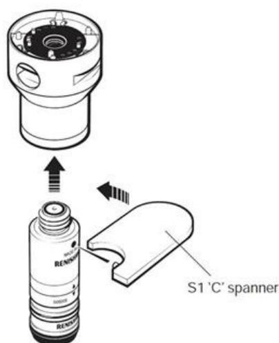
The S1 spanner is designed to fail before damage can occur to the mechanical joint between the two parts. Using the S1 spanner, fully hand-tighten the probe body into the M8 bush (0.3 Nm to 0.5 Nm).
