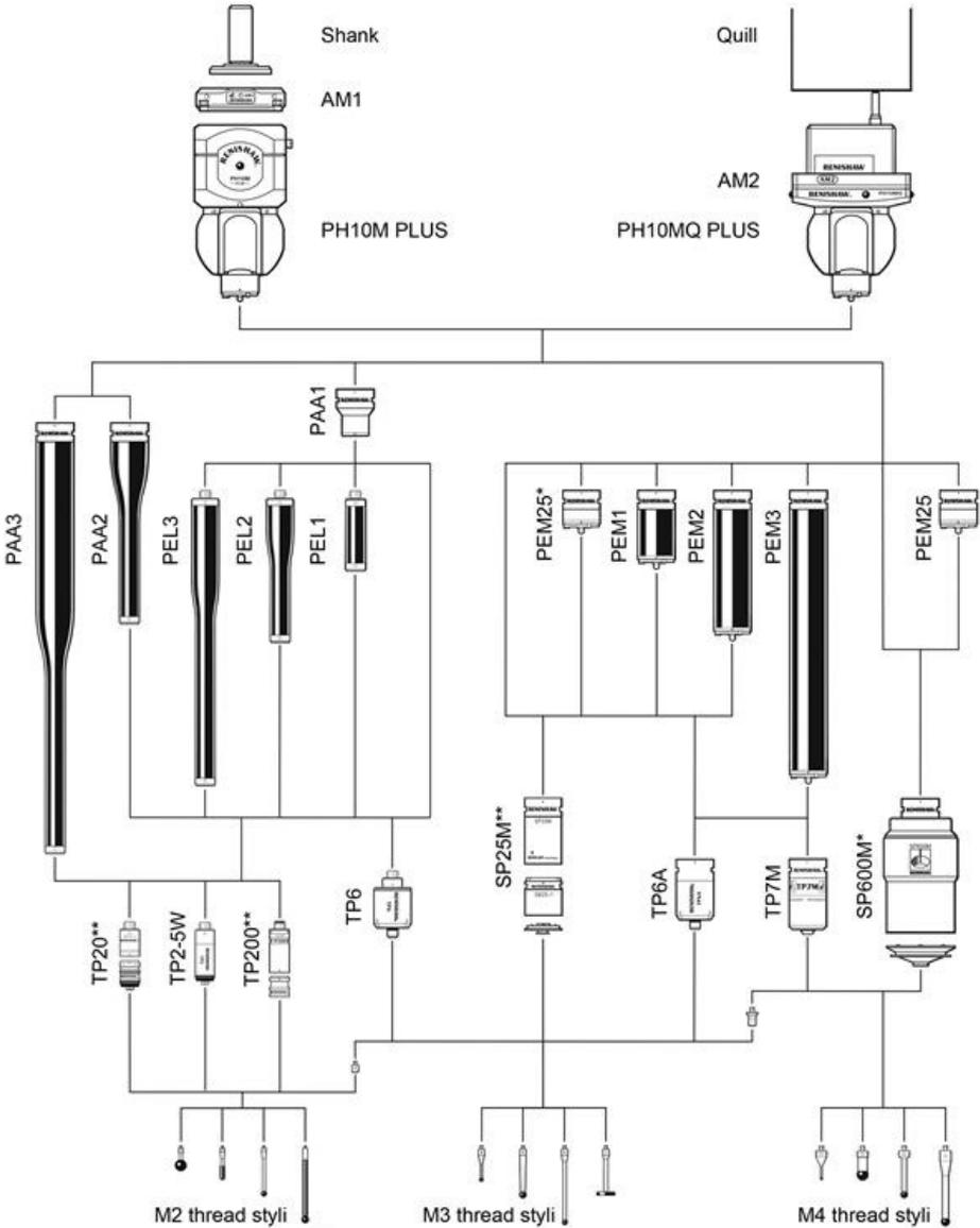
\* PH10MQ PLUS used with SP600M requires a PEM25 extension bar to achieve A = 97.5° or A = 105° in all B-axis positions.
