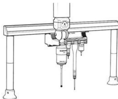
ACR3 is a passive modular autochange rack with four ports and is driven by the motion of the CMM. Two ACR3s can be linked to provide an eight port system. The ACR3 is mounted on the horizontal Renishaw MRS (modular rail system).
