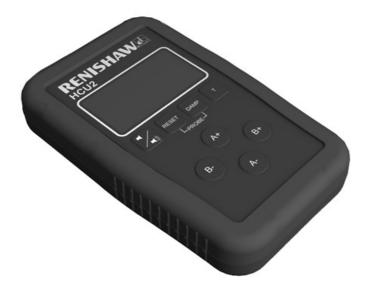
HCU2 enables the probe head to be used in a manual mode and is invaluable for component set-up, operator-controlled inspection and teach cycle programming. HCU2 has a two-speed action, with a choice of jog or sweep moves. The LCD screen provides head angle and system status information as well as error analysis.
