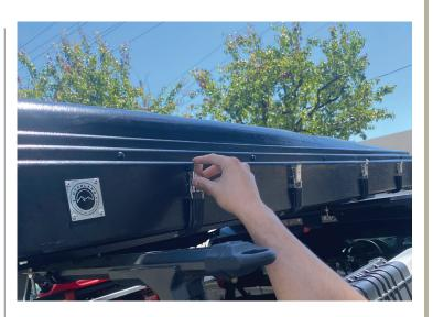
**6.** Pull down the straps, and securely fasten the fastening clips and reinforced straps.
