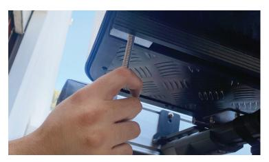
**3** Have a friend lift the Bushveld while a second person slides the piece over the crossbar so that one bolt is on each side of the bar.
