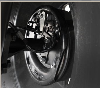
MANUAL PARKING BRAKE WITH ELECTRIC 10" DRUM BRAKES
