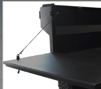
ELECTROSTATIC PLATED AND MILITARY GRADE TWO-STAGE BLACK POWDER COATING FINISH
