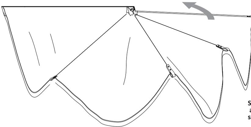
Swing out left arm fully and attach to roof rack using supplied tension strap
