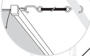
Swing out left arm fully and attach to roof rack using supplied tension strap
