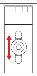
NOTE: Make sure there is spacing between interior cap lip and female clamp portion to prevent damage
