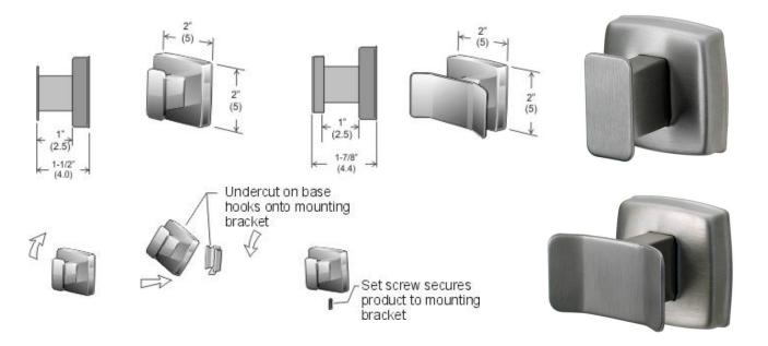
**Mounting of Product:** Screw concealed mounting system: The mounting bracket is attached to the wall with screws at the desired height. The unit is then hooked onto the bracket. When the set screw is tightened the product is firmly secured to the wall. The set screw applies pressure to an inclined surface on the bracket this provides a rattle free and integral mounting of the product. (mounting bracket and screws provided).
