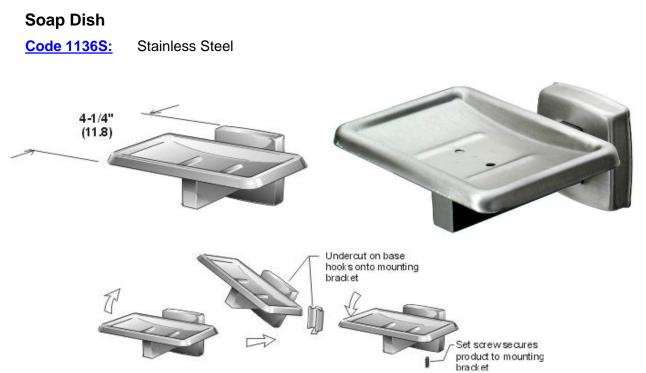
**Mounting of Product:** Screw concealed mounting system: The mounting bracket is attached to the wall with screws at the desired height. The unit is then hooked onto the bracket. When the set screw is tightened the product is firmly secured to the wall. The set screw applies pressure to an inclined surface on the bracket this provides a rattle free and integral mounting of the product. (mounting bracket and screws provided).
