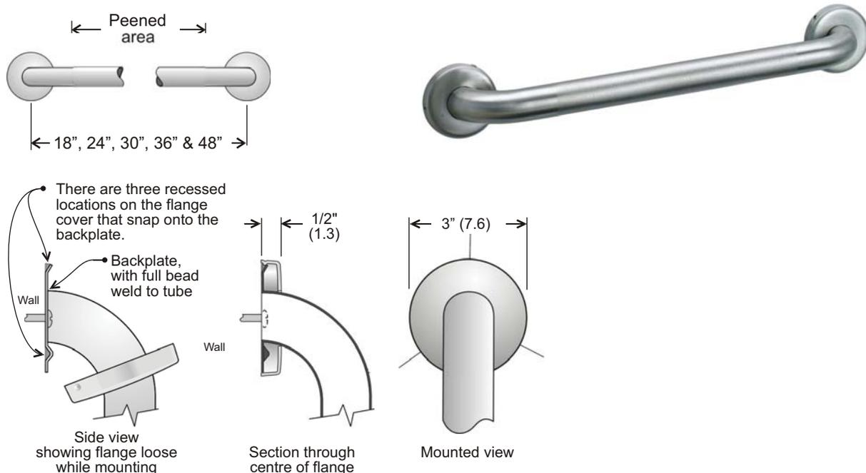
Concealed mounting screws, using snap flange, on "SP & NP" codes
