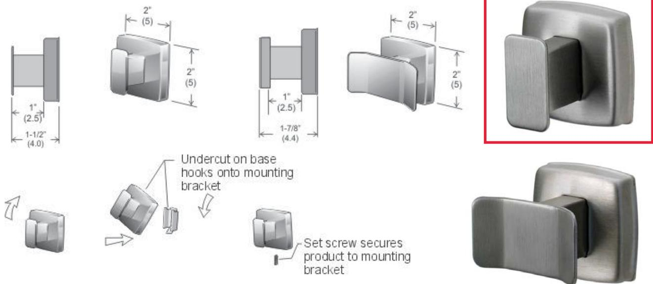
**Mounting of Product:** Screw concealed mounting system: The mounting bracket is attached to the wall with screws at the desired height. The unit is then hooked onto the bracket. When the set screw is tightened the product is firmly secured to the wall. The set screw applies pressure to an inclined surface on the bracket this provides a rattle free and integral mounting of the product. (mounting bracket and screws provided).
