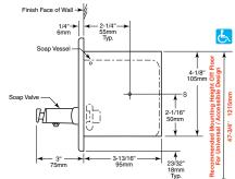
Rough Wall Opening 8-3/8" (210mm) wide 4-3/8" (110mm) high 3-7/8" (98mm) minimum recessed depth
