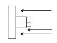
6. With the slots in the tube facing down, pass the thread of the bolt (M8 Hex Screw) through the slot in either end of the tube from the inside. Hold the tube and gently twist to help the bolt (M8 Hex screw) pass through the slot. Repeat for other end of the tube while keeping the slots facing down to avoid losing the part just fitted. Make sure the shape of the half-moon washer is aligned with the inside diameter of the tube.
