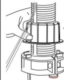
10. Connect larger diameter tube from the Stem Mixer Housing (Parts List: Item 11) on to barb of Retainer located on top.
