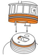
13. Insert Bottle with Gasket, Washer, and Gasket to the Adapter ensuring prongs go in appropriate holes in the bottle.
