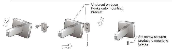
Screw concealed mounting system: The mounting bracket is attached to the wall with screws at the desired height. The unit is then hooked onto the bracket. When the set screw is tightened the product is firmly secured to the wall. The set screw applies pressure to an inclined surface on the bracket this provides a rattle free and integral mounting of the product. (mounting bracket and screws provided).
