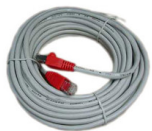
PATCH CABLE/ CROSS OVER/ RJ45-RJ45/ CAT.5/ L=10M/ GREY/ 4X2X0.14MM2/ WITH FOIL SHILDING AND ANTI KINK BUSH/ 100MHZ PATCHKABEL/ CROSS OVER/ RJ45-RJ45/ KAT.5/ L=10M/ GRAU/ 4X2X0,14MM2/ MIT FOLIENSCHIRMUNG UND ROTER KNICKSCHUTZTÜLLE/ 100MHZ 75120025
