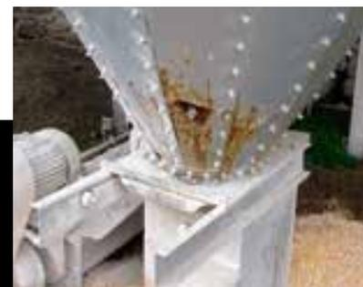
**Is the bottom of your tank rusting out? Hopper extension kits allow you to replace the bottom of the hopper section instead of replacing the entire tank.**
