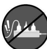
Prevent the power cord from being damaged by pressure or excessive bending.
