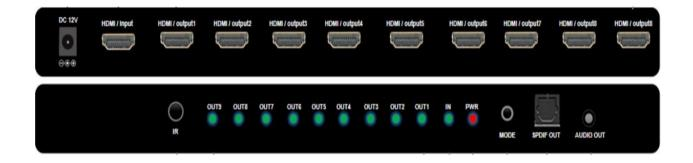
This **WolfPack 4K 30 Hz 1x9 Video Wall Controller** supports 1 HDMI input and 9 HDMI outputs, and its main function is to divide a complete HDMI high-definition image signal into 9 blocks and distribute them to 9 video display units (such as rear projection units, LCD TVs, etc.), to create a dynamic image large screen with 9 HDMI high-definition video display units.
