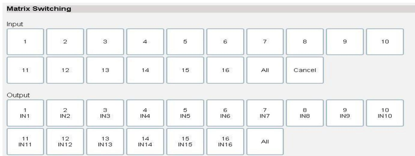
The web interface switching method mirrors the device panel operation: first select the input source, then select the output channel for instant switching.
