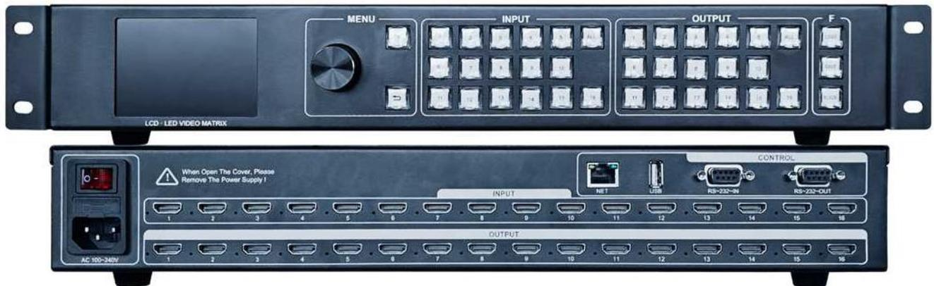
The **HDTV16x16AMSMTX** is a seamless switching matrix that supports 4K input and output, offering flexible management of multiple signals. It supports a maximum resolution of 3840×2160@30Hz and features a built-in MEAN WELL power supply, crystal buttons, and a full-color LCD screen for easy operation. The device can be controlled through various methods, including panel buttons, a web-based interface, serial port protocol, and more.
