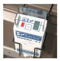
Your Bed-Check Model Vr is now ready to monitor your fall risk individual as soon as the Sensormat pad is properly placed and connected, and the nurse call system is connected (if used).
