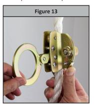
**Step 7:** Connect the SAL to the arrestor (if applicable).
