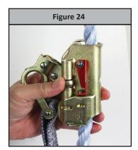
**Step 6:** The 8355 Fall Arrester is permanently connected to a SAL equipped with a self-closing and self-locking snap hook. Attach the snap hook to the dorsal D-ring of the FBH.
