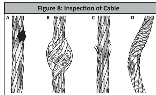
Extract all of the cable and check the entire working length for damage caused by chemical corrosion or excessive heat as evident by discoloration (A), bird caging (B), broken wire strands (C), kinks and bent strands (D), see Figure 8. The cable should retract completely without faltering and should remain taut under tension without sagging.
