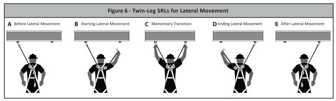
Avoid sudden or quick movements during the normal work operation, as this may cause the SRL pawl system to engage and possibly cause loss of balance, which may cause injury or death. If a fall occurs, the pawl system will engage and lock the lifeline. The EA will deploy to arrest the fall and limit arrest forces on the user.
