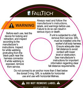
!INSPECTION! Inspect this product before each use. Semi-annual inspection by a competent person is required. Do not use if inspection reveals unsafe or defective condition. Remove the product from service immediately if it has been subjected to fall arrest forces. See the user instruction manual for complete inspection procedures.
