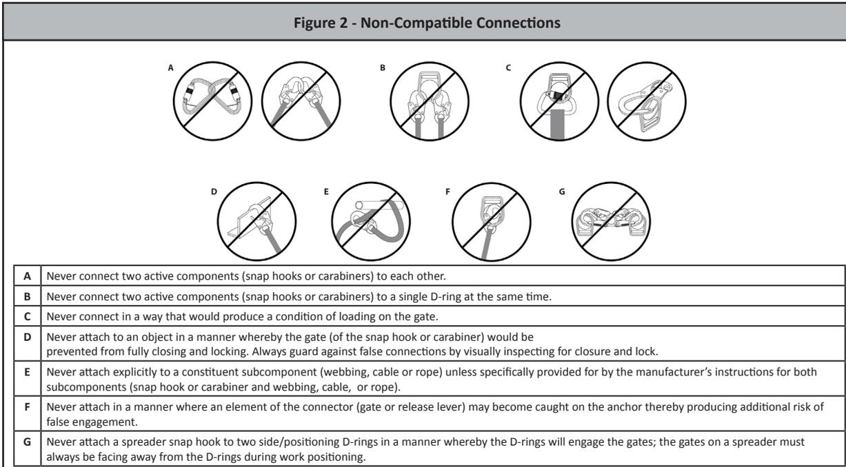
**4.3 Compatibility Of Components:** This equipment is designed for use with approved components and subsystems only. Substitutions or replacements made with non-approved components or subsystems may jeopardize compatibility of equipment and may affect the safety and reliability of the complete system.
