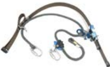
Figure 24: WPFRD Initial Position
