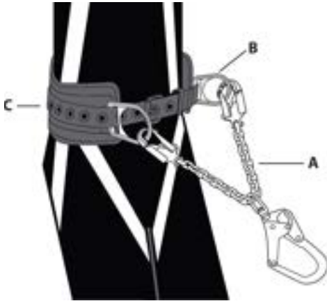
Figure 6 - Correct Attachment to Side D-Rings
