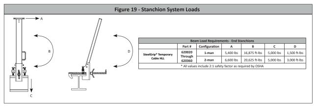
Note: The maximum single span length when using stanchions is 60', see Figure 20. The overall system length can be increased by using intermediate stanchions to create multiple spans in at most 60' increments. For multiple spans two FallTech SteelGrip® Coil Energy Absorbers must be used, see Figure 21.
